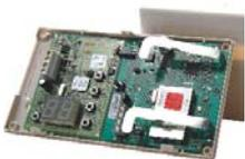
This input expander enables wireless inputs to be added to control panels in the EURO MERiDIAN range. Depending on its mode of operation, it will accept signals from 7 or 29 wireless transmitters. Assigning the devices to individual zones is simple and the signal strength is displayed for each transmitter.
